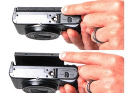
The LCD screen on the back of the SX730/SX740 camera is hinged.
