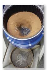
Wires are mechanically polished in a proprietary media with an abrasive polishing agent ensuring the best wire surface for optimal sliding mechanics during clinical treatement.
